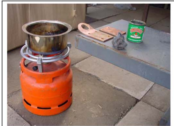
All connections are tinned – Picture shows Steel wool, tower copper connection, flux and a stove for melting Tin.
